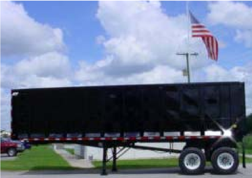
30 Foot Quarter Frame Trash Trailer with square front bulkhead, high side walls, optional AR-400 floor and rugged rear doors.
