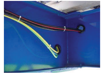
Color coded air hose and grommet lined frame holes are standard
